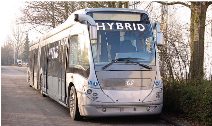
The Phileas Hybrid bus combines an electric powertrain with a CNG, LPG or diesel one
