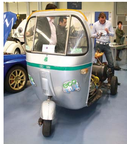
The LPG powered eco tuk features a two-stroke engine with Direct Injection technology
