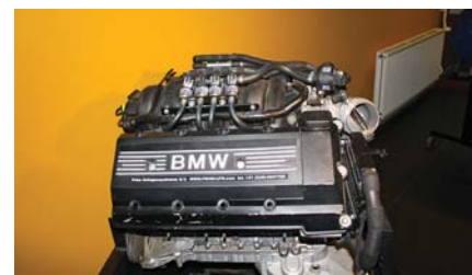
A BMW M5 powertrain fitted with a Prins VSI kit
